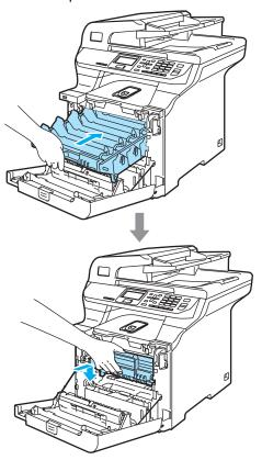
Insert the original orange packing material for the drum unit until as shown in the illustration, and then close the front cover.
